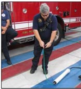
Simply inflate the plug until the leak is stopped....
