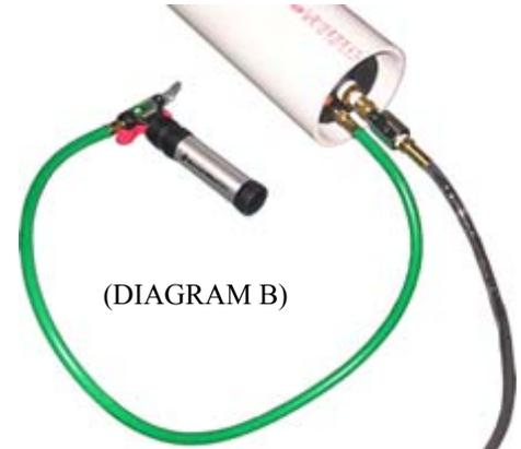
If too much head pressure is present and the plug is being forced out of the pipe, just simply open the shut-off valve to relieve the pressure (see diagrams A & B)
